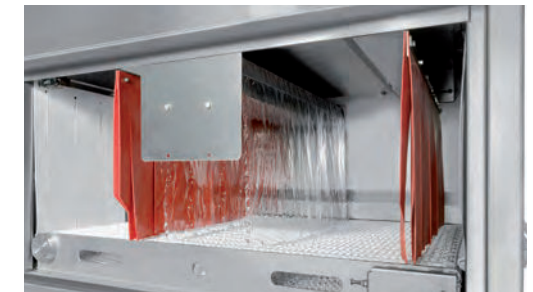
Two water curtains from above and two water nozzles from below.
