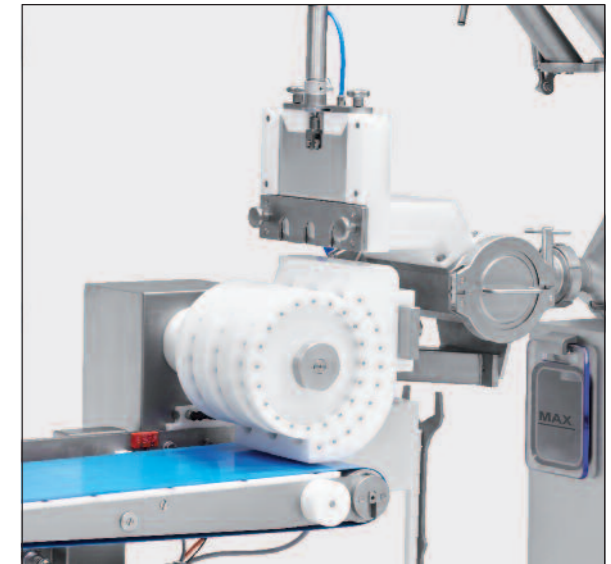
High performance thanks to multi-row form rollers
