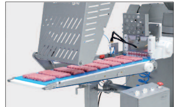
Cevapcici shaping by flow divider & form cutter
