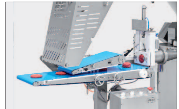
Cevapcici shaping by flow divider & form cutter
